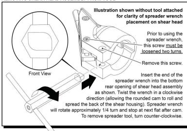
SERVICE TOOLS: Spreader Wrench No. 61-30-0300 for 14 Gauge Shear Head used on Shear
